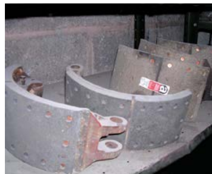
Figure 41 Asbestos brake linings for quarry vehicles
